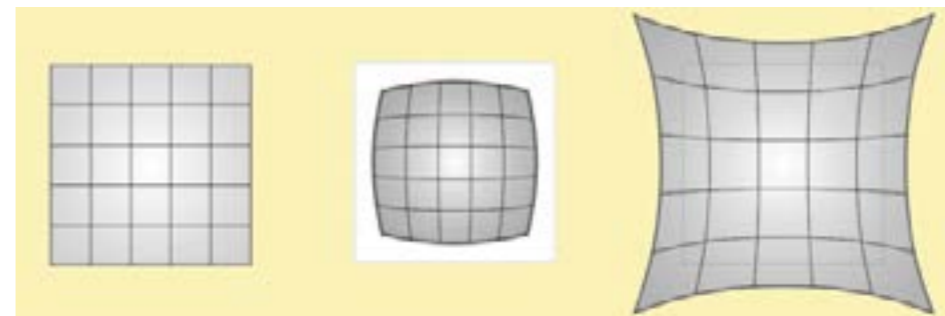
Distortion: Distortion depends on the location and the angle of the camera sensor relative to the object. This must be taken into consideration in the case of objects that are located at different positions in the image area. Distortion-free image (left), barrel distortion (center) and pincushion distortion (right). (Image: ipf electronic gmbh)
