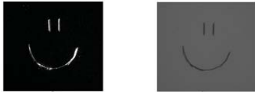
Scratches on a Plexiglas pane. Left: With dark-field transmitted light illumination, the artifacts stand out as bright areas. Right: Bright-field transmitted light illumination.
