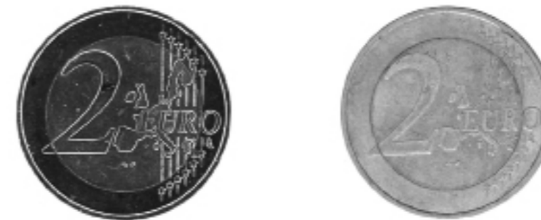
Picture of a 2-euro coin with dark-field illumination (left). For comparison, the coin with bright-field illumination (right). With dark-field illumination, the engraving on the coin stands out from the background with high contrast.
