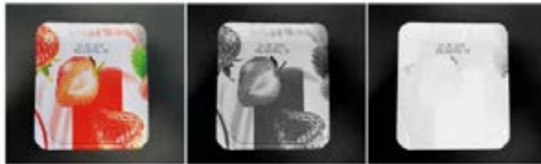
Color photo (left) and photo of a yogurt cup with a monochrome camera under white light (center). With infrared light, the colored design is nearly completely suppressed with the exception of the black writing (right).
