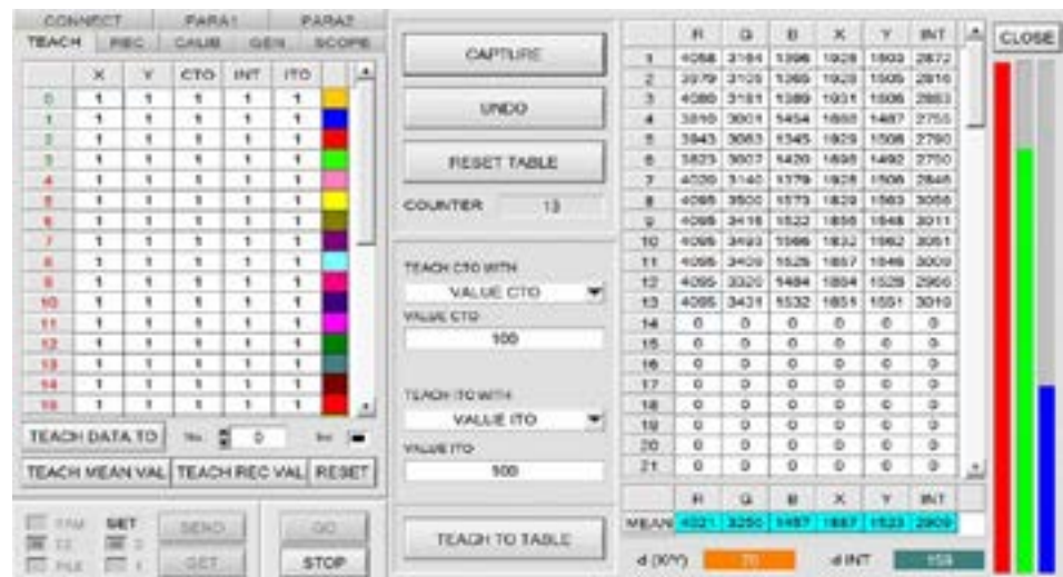
In the case of difficult surfaces, one special characteristic of ipf electronic color sensors is their ability to determine reference or target values by averaging one or more good components over several target surface points. (Picture: ipf electronic gmbh)
