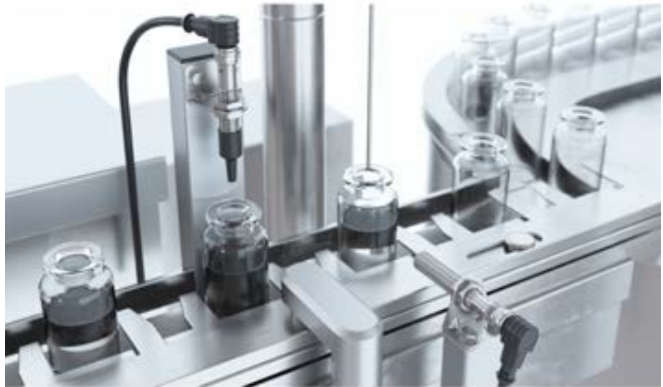
Level control and presence control with two ultrasonic sensors at a dosing station.
