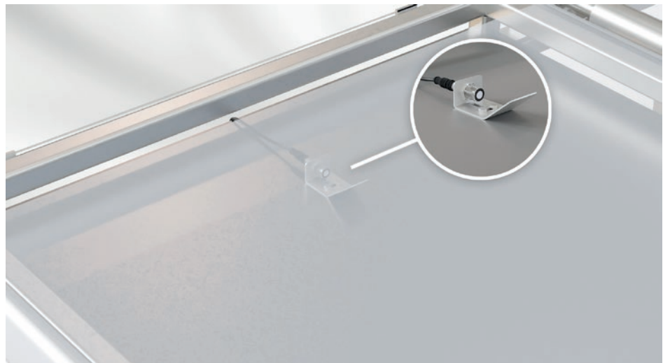
An ultrasonic diffuse-reflection sensor UT189523 for checking the presence of film. A mounting bracket with deflection function directs the ultrasound in the direction of the object to be detected and enables installation below the film despite the limited installation space. The sensor is also protected from potential contamination in this installation position.
