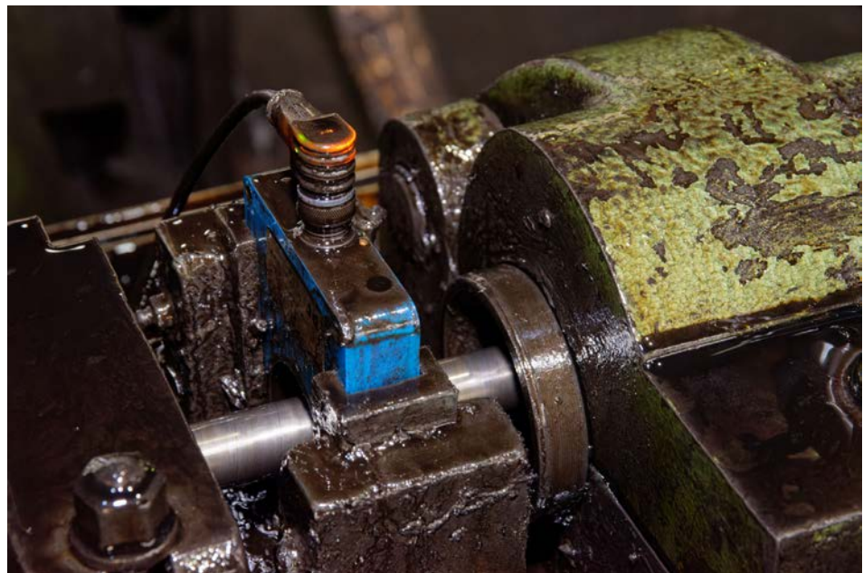
The IY500320 inductive ring sensor always works reliably even in extremely oily environments and reliably detects the round steel at the cut-to-length machine.
