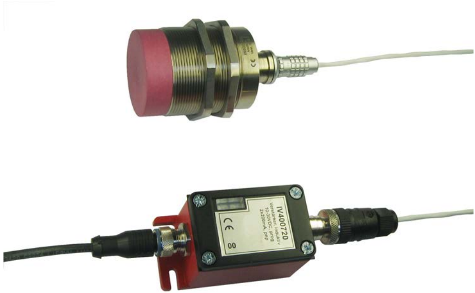
The IN50C543 inductive sensor of the two-part system ( IV400720 amplifier below) for position sensing of a lifting device in a baking oven withstands temperatures up to +230°C.
