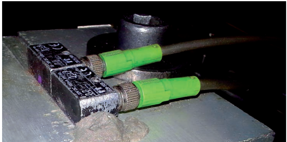
High temperatures up to +100°C and extraordinarily high mechanical loads. MZA70155 cylinder sensors are exposed to high temperatures up to +100°C and extremely high mechanical loads.
