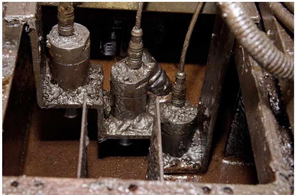
FK920420 capacitive level sensors in a storage tank for permanent lubrication of a punching tool.
