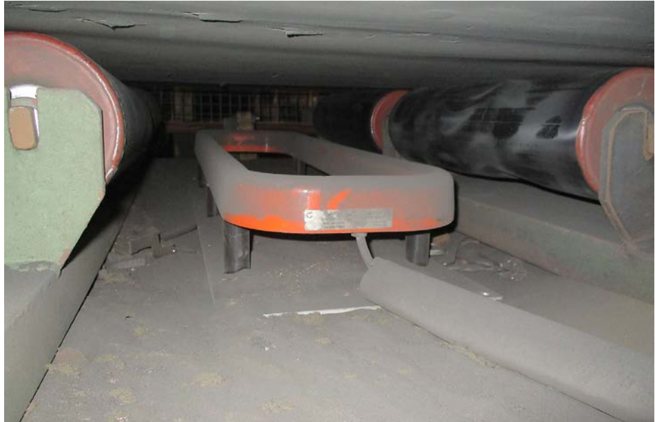
The detector coil works perfectly even if, over time, dirt and metal dust are deposited on it (All images: ipf electronic gmbh)
