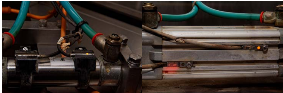
Robust and extremely durable: The MZR401A9 (top) and MZ0701A8 cylinder sensors in metal housings replace conventional devices made of plastic in a filling line, as these were not able to withstand the frequent cleaning cycles with an alcohol-based cleaning agent and therefore had to be replaced more frequently.
