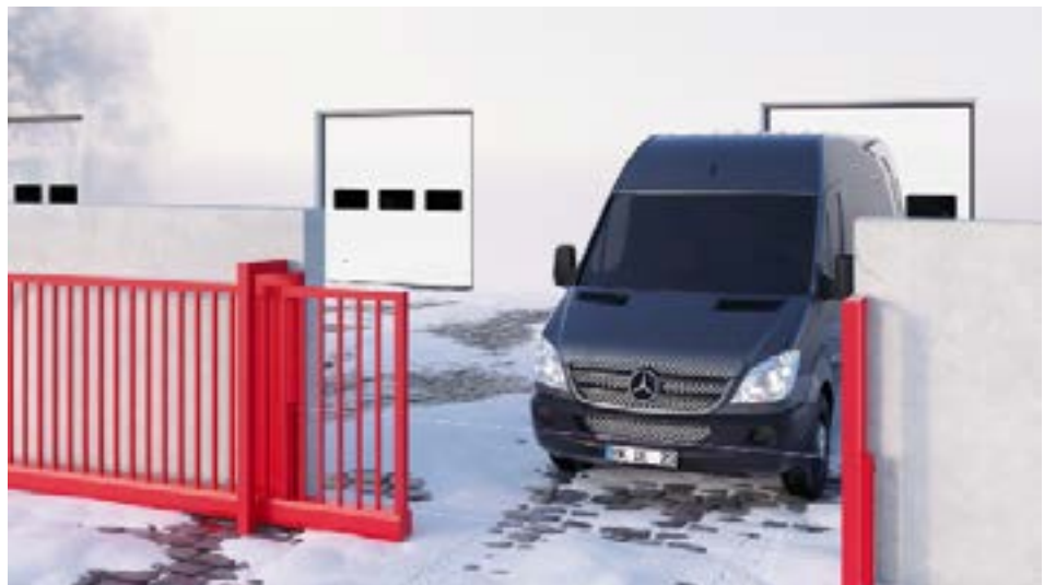
Light barrier with multiplex amplifier (2-channel) at a gate entrance. The system works perfectly even if the snow on the ground protrudes into the lower infrared beam, as the specified transmission power is automatically readjusted.
