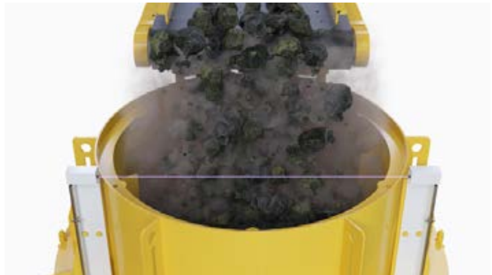
Light barrier with single-channel amplifier (manual operating mode) for overfill protection on a rock crusher. The material flow does not trigger a switching function during refilling.
