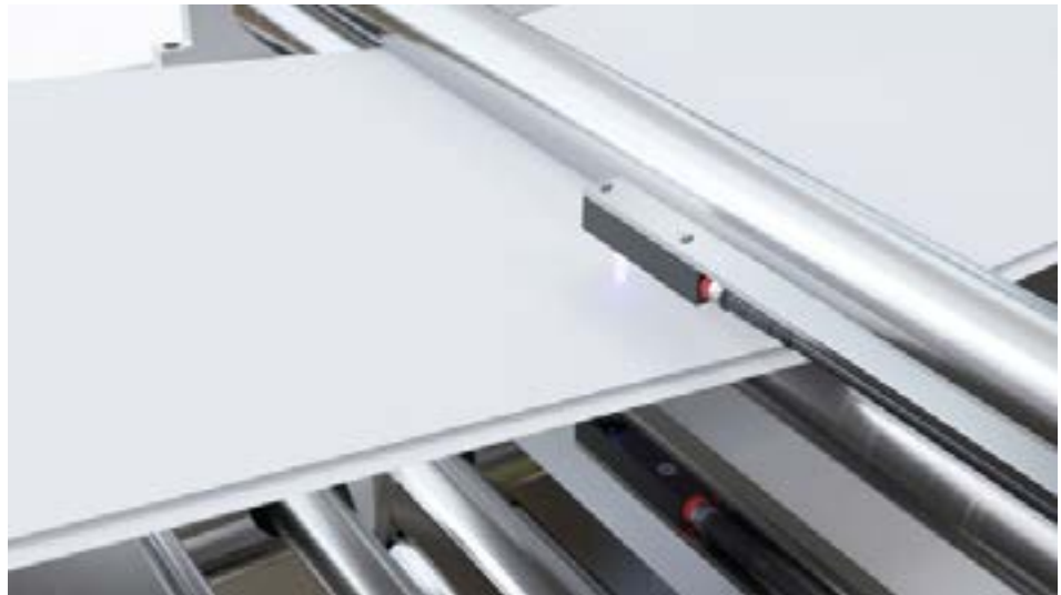
High-performance light barrier with single-channel amplifier in measuring mode for double layer control. The number of material layers can be precisely determined via the analog output.
