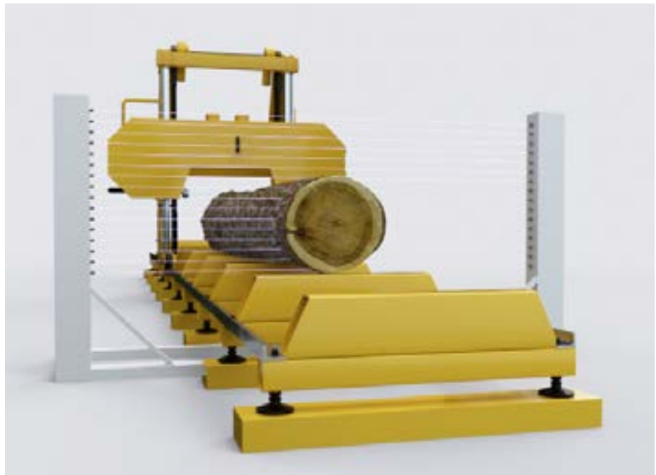
Light grid on a conveyor belt for logs in front of a band saw. By coupling several multiplex amplifiers, solutions with flexible light grid height can be realized.
