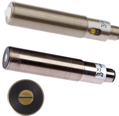
Laser system with soiling compensation (top: PE180122 receiver; bottom: PS180022 transmitter). For special measuring tasks, the light beam is focused by means of slit diaphragms integrated in the transmitter and receiver.
