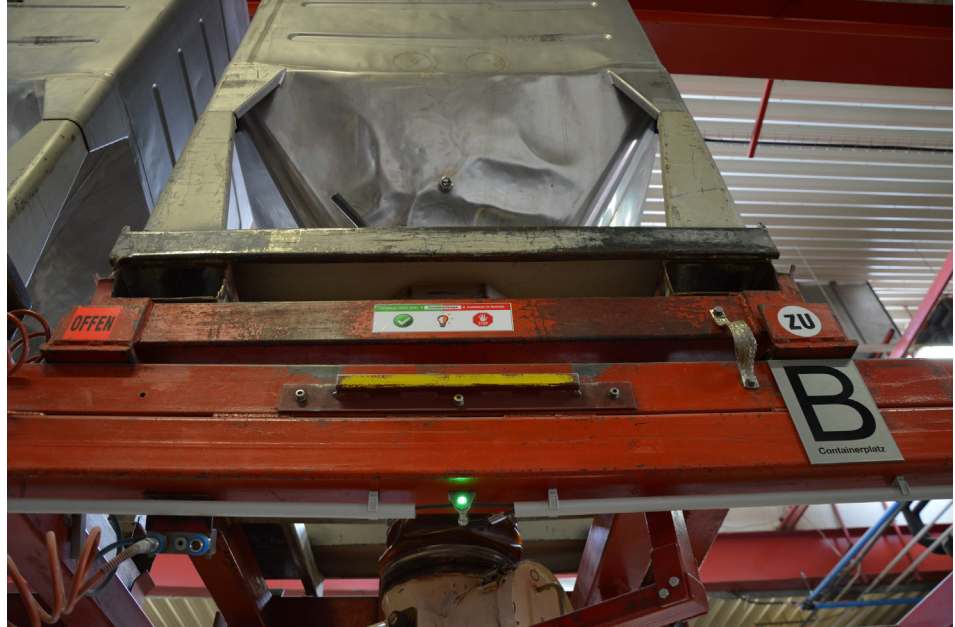
Simple, compact and effective solution: The LED bicolor lights are located below the raw material containers. A green light signals the raw material container to be replaced to the forklift driver.
