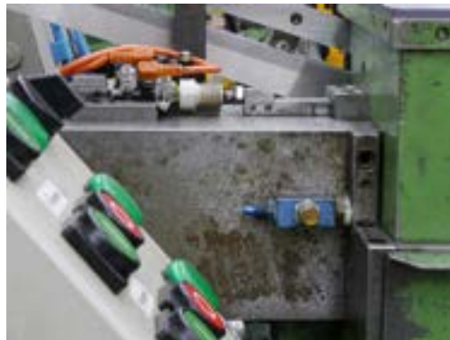
Two very compact sensors on an extremely short pneumatic cylinder.
