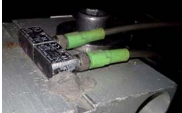
Magnetic cylinder sensors on a special hydraulic cylinder. The sensors must with-stand very high mechanical loads and temperatures of up to +100°C.
