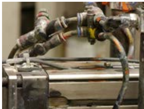
The sensors even withstand paint splatters, dried-on paint residues or cleaning agents and solvents.
