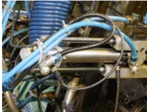
Cylinder sensors in an extremely oily environment on a machine.
