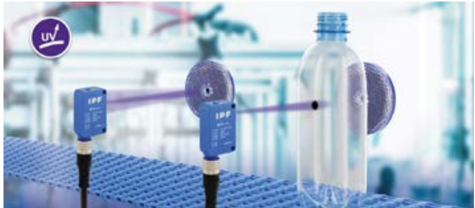
The retro-reflective sensors are all but predestined for use in high-speed processes due to their high switching frequency of \leq 1\text{kHz} . This is a typical example from the beverage industry, with the detection of transparent PET bottles.
