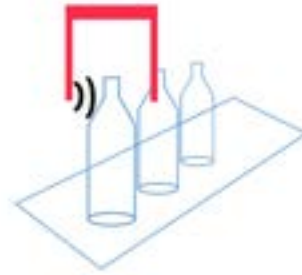
The detection of glass or PET bottles with an ultrasonic fork.
