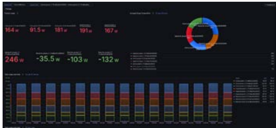
Display of active, apparent and reactive power of a system with distribution terminal of the respective phases (L1, L2 and L3).
