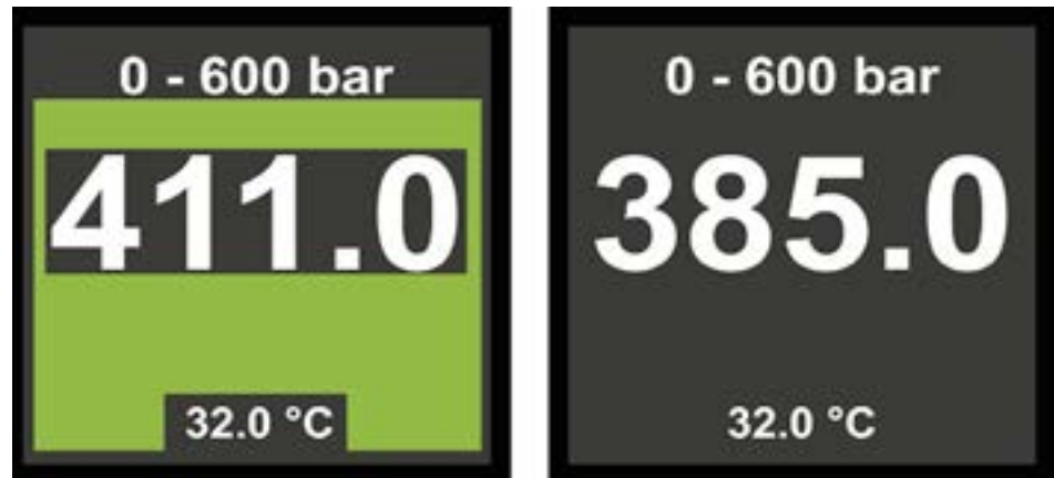
Example of the current status of a switching output: switching output active (left), switching output inactive (right)
