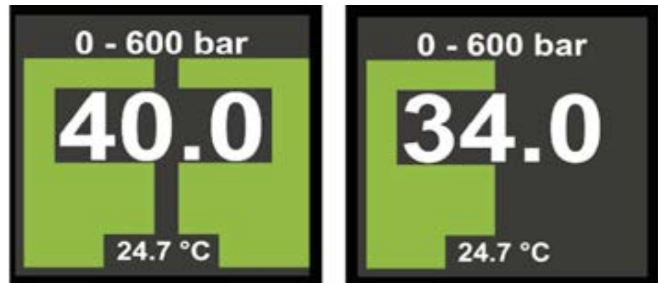
Example of the current status of two switching outputs: Both switching outputs active (left), switching output 1 active - switching output 2 inactive (right)
