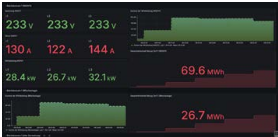
Current measured values from a counter for a specific operating range for voltage, current, active power as well as total active energy and total active power of a system are clearly displayed on the dashboard.
