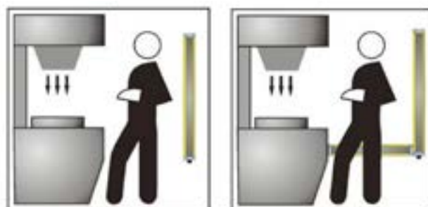
Fig. 13: Installation of a safety light curtain with resolution for body protection: incorrect installations are shown at the left, as the person can pass between the ESPE and the machine to enter the danger area; at the right, a horizontally installed safety light curtain reliably safeguards the danger area.
