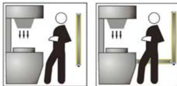
Fig. 13: Installation of a safety light curtain with resolution for body protection: incorrect installations are shown at the left, as the person can pass between the ESPE and the machine to enter the danger area; at the right, a horizontally installed safety light curtain reliably safeguards the danger area.
