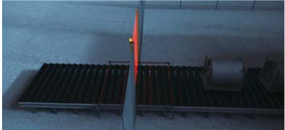
Fig.10: With muting, the protective function of a safety light curtain can be automatically deactivated for a short time in order to transport conveyed material into a protected area.
