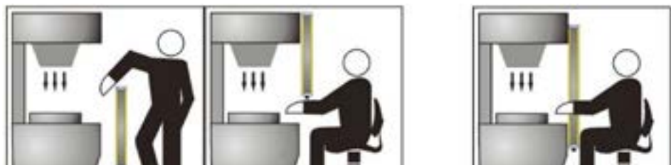
Fig. 12: Installation of a safety light curtain with resolution for hand protection: incorrect installations are shown on the left, as the person can both reach over the safety light curtain and well as place a hand underneath to enter the danger area without triggering the ESPE. The correct installation is shown on the right.
