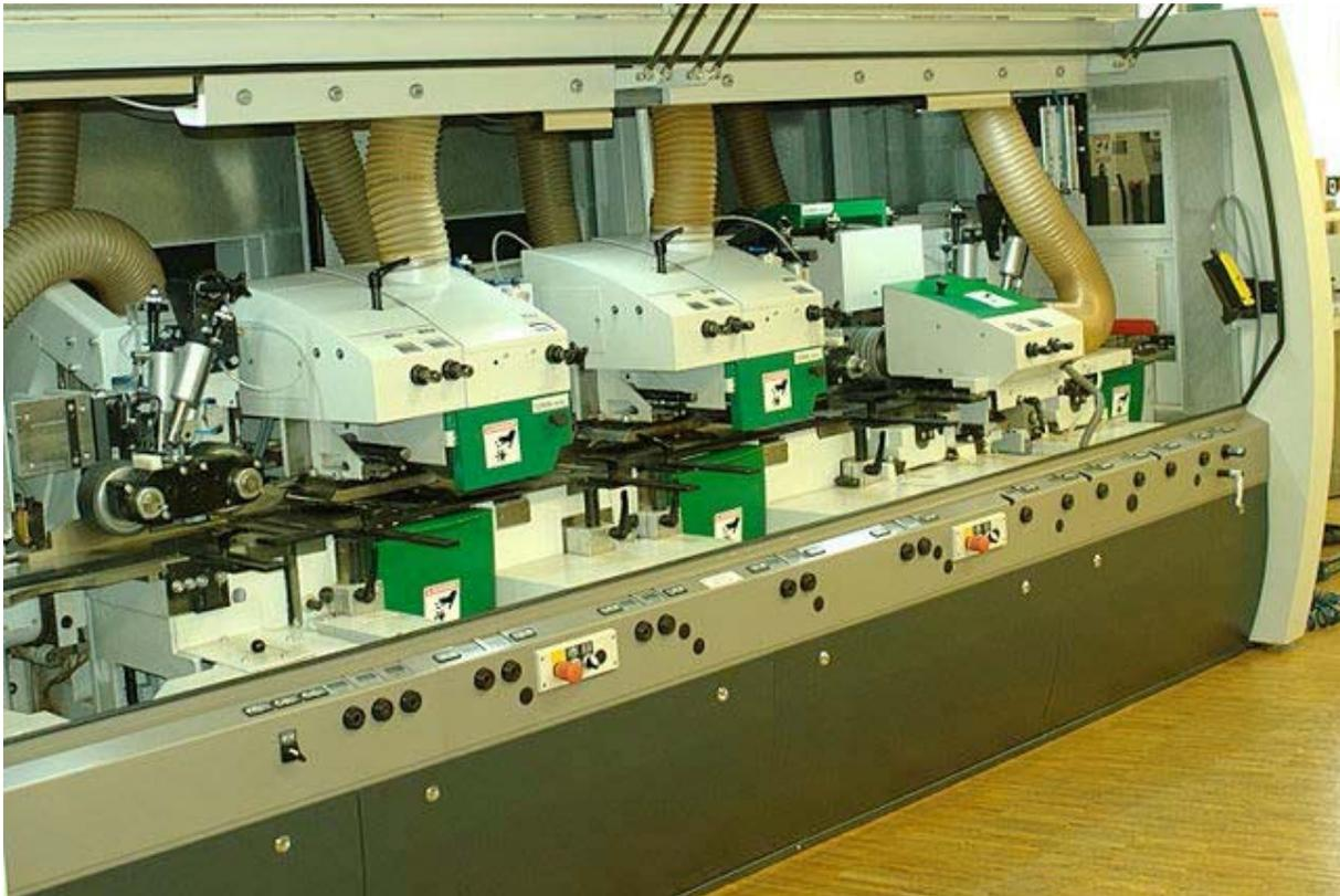
*Different frequencies have to be evaluated for the spindle drives of the different drives: Up to 70Hz in the case of standard machines, up to 300Hz in the case of high speed aggregates and up to 800Hz in the case of high speed spindles.*
