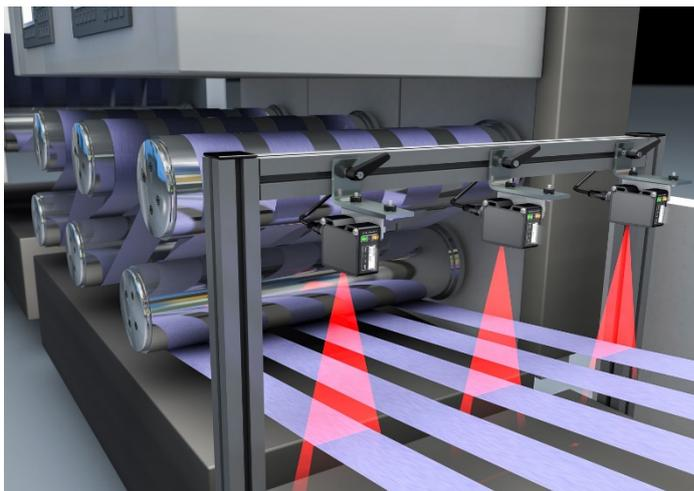
The light section sensors were installed above the bitumen sheet that has to be monitored.
